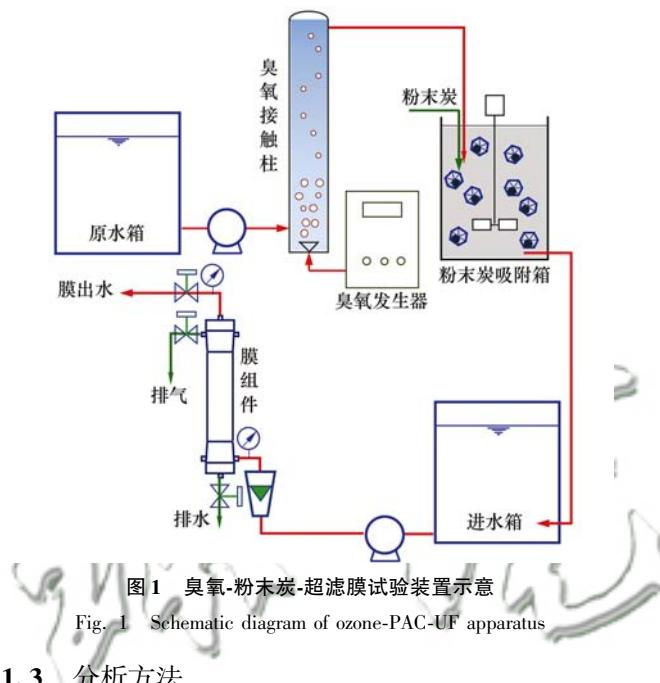
Fig. 1 Schematic diagram of ozone-PAC-UF apparatus
