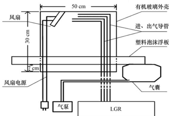
图 2 Schematic diagram of the floating chamber
